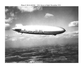
What I had seen was the U.S. Navy dirigible U.S.S. Akron, the largest airship every built. It was 785 feet long, 132 feet in diameter and 152 feet high, cruising speed of 55 knots and range of 5940 nautical miles, a flying air craft carrier that could store up to five airplanes and launch and retrieve them while in flight. I saw it fly over Miami while launching and retrieving 3 of its airplanes.
